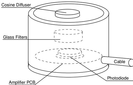
The DET201450 detector comprises of an aluminium housing, photodiode, R450 filter and PCB assembly.
